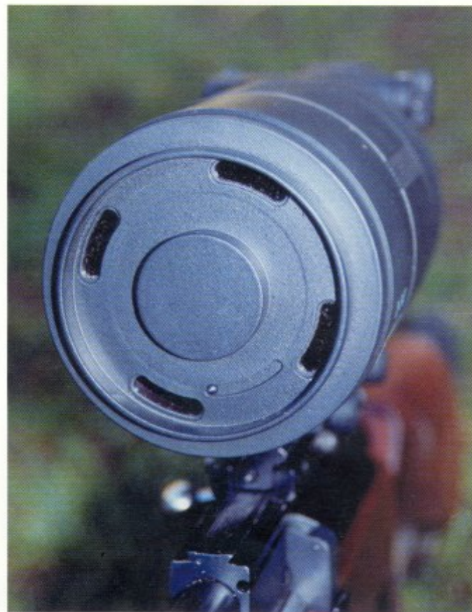
A night scope pinhole lens cover – this unit rotates, opening up small slots which allow the unit to be zeroed in daylight
