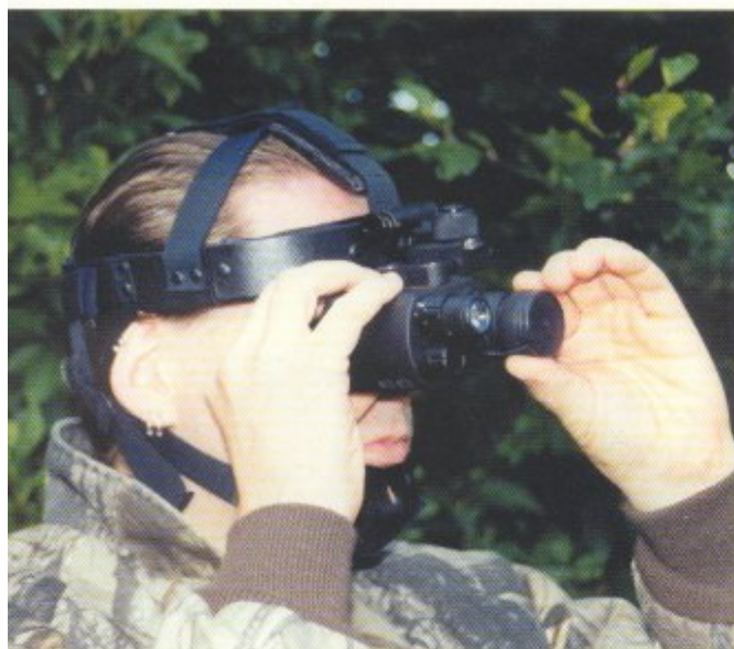
Monoculars can be worn on a head harness, leaving the hands free
